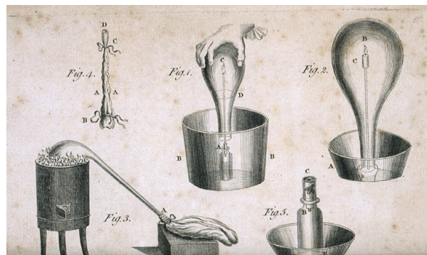
Scheele's diagrams for the collection of, and experimentation with gas. The gas-bags used to collect the gas, Fig, 3 and 4 in the diagram, were formed from animal bladders tied off at the ends.
