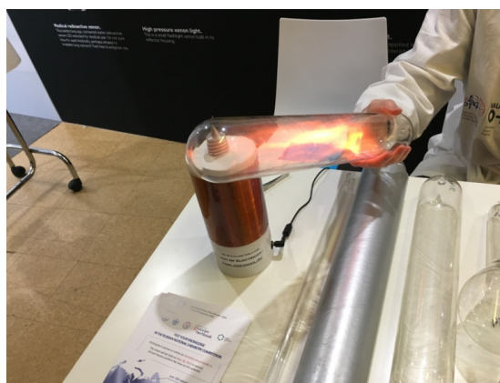
Gas discharge tubes with gases trapped and excited by a Tesla Coil (NEON)
