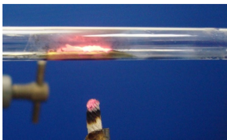
Figure 3: Reduction of copper(II) oxide with hydrogen
