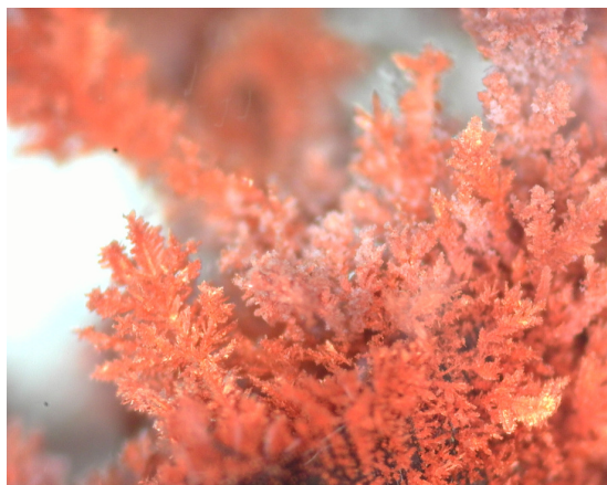
Figure 17: Copper crystals forming at the cathode during electrolysis. This was taken with an expensive Dinolite USB microscope ( http://www.gtvision.co.uk ).
