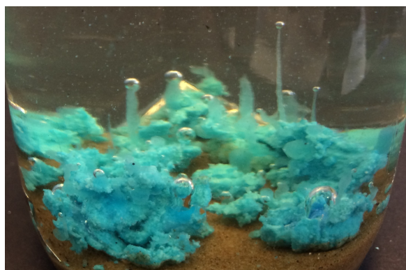
Figure 2: Copper (II) sulfate in water glass solution
