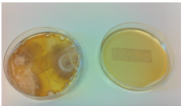
Figure 3: Experimental result of a cream-agar patch test after 10 days. Right side: paraben-containing cream, left side: paraben-free cream.
