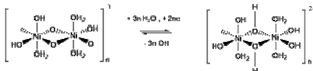
Scheme 3: Topotactic redox reaction in hydrated layer in hydrous nickel oxy-hydroxide.
