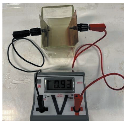
Figure 3: Simplified version of Voltaic Pile with sulphuric acid as the electrolyte.
